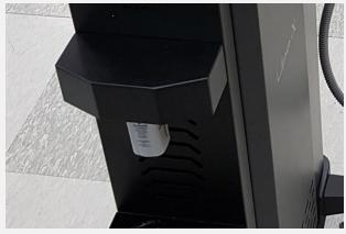
Alcohol passed through the tube is held in the filter on the back of the machine. Turn the filter counterclockwise to open, discharge the contents and reeuip.
