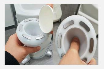
Start the RF-vacuum and pour in some alcohol little by little into the hole. Ant block the hole intermittently to soak up. Repeat 3~4 times.
